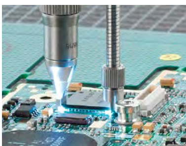
ERSASCOPE 2: exchangeable optics for CSPs
