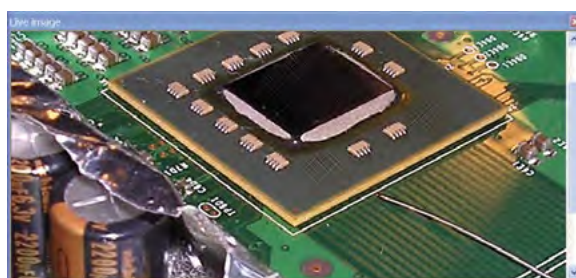
Rework process visualization with live image window
