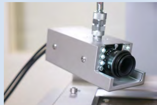
Reflow process camera on the HR 550
