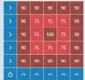
Full-size heating with edge enhancement and "hot spot".
