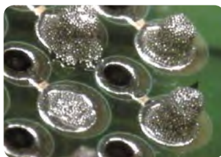
BGA – paste print: insufficient solder
