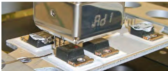
TO220 on aluminium carrier with hybrid rework system
