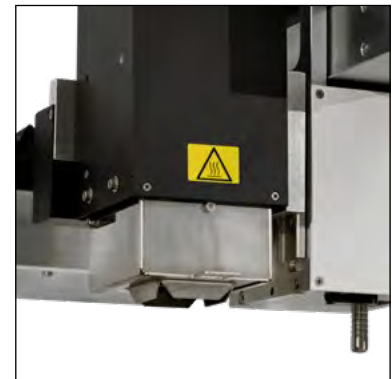
Hybrid heating head with interchangeable adapters
