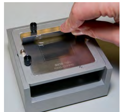
Flux deposition in the dip stencil
