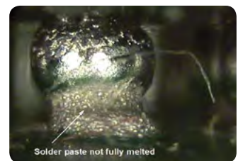
PBGA – scaling: insufficient heat
