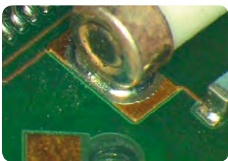
Lead-free assembly: non-wetting
