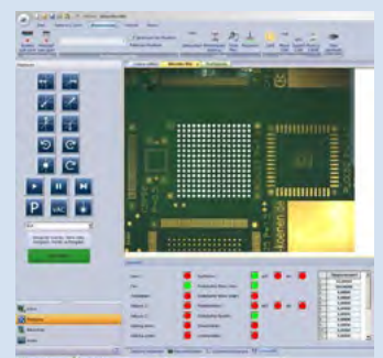
Superimposing of component and target position
