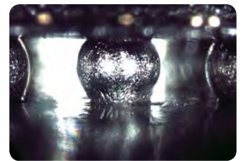
PBGA – cold joint: insufficient heat
