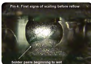
PBGA – scaling: insufficient heat
