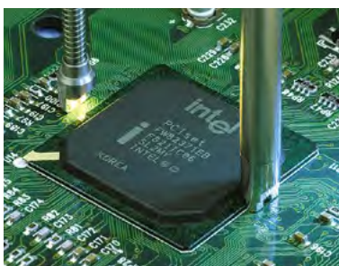
ERSASCOPE 1: fixed optics for BGAs
