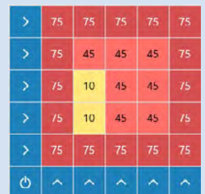
Full-size heating with edge enhancement and "cold spot".
