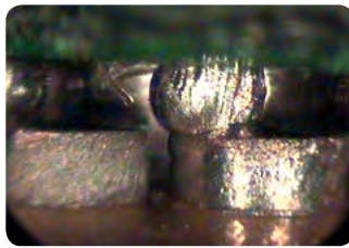
BGA – piggy back: bad alignment
