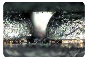
PBGA – scaling: insufficient heat
