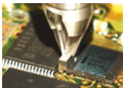
Small footprint of Flip Chip lens: 0.6 mm x 4.0 mm
