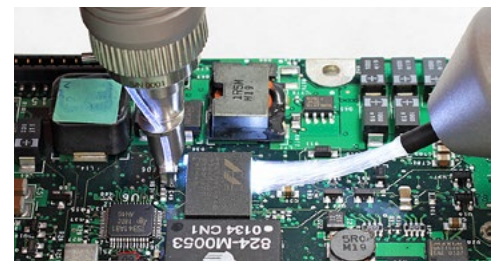
Inspection of a micro-BGA
